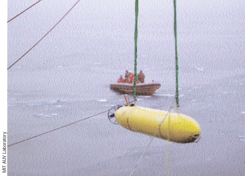
Figure 6. A Dorado autonomous underwater vehicle on field trials in the Arctic Ocean in late 2001 for the Monterey Bay Aquarium Research Institute.
