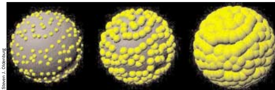
Figure 2. Metal nanoshells—composite layered nanoparticles whose color is determined by controlling the thickness of the layers—are being developed in a collaboration between the Rice Quantum Institute, the Halas Nanoengineering Group, and the physics and bioengineering departments. Here we see the growth stages of gold shells around silica nanoparticles.
