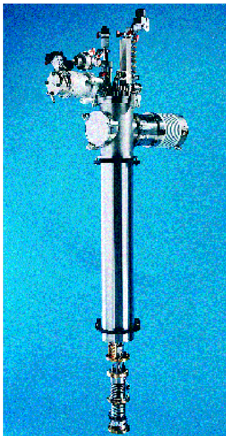
A dilution refrigeration insert for operation below 10mK, with turbomolecular pumps
